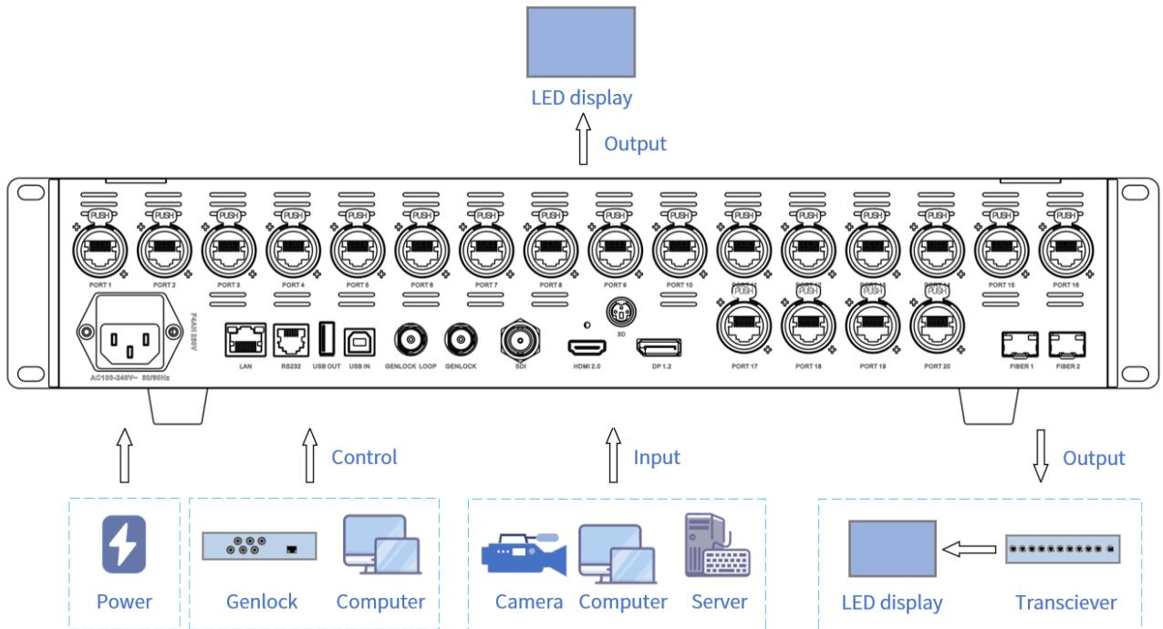
**Network port output:** When selecting the network port output, you can connect to the LED display through the network cable.
